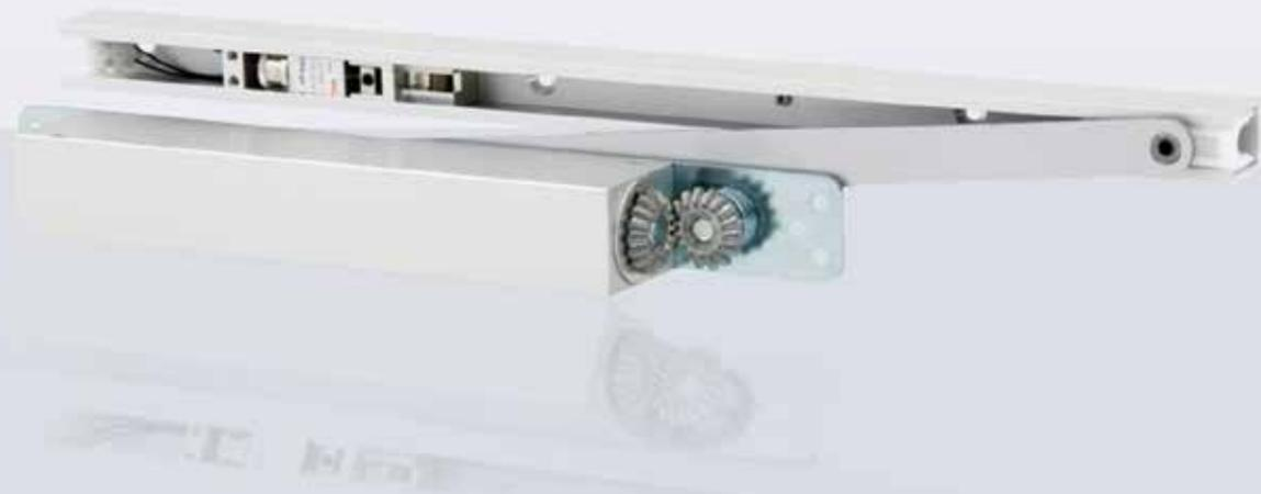
The beauty of the Lockwood Concealed Door Closer Systems is that they stay virtually invisible when the door is closed, keeping your design pure and clean just as you intended. Featuring efficient 'cam action' technology, it has an in-built power adjustment mechanism which allows you to reduce opening force whilst maximising closing force, making it perfect for almost every new door design. When it's all about aesthetics, the Lockwood Concealed Door Closer Series is the best choice.
