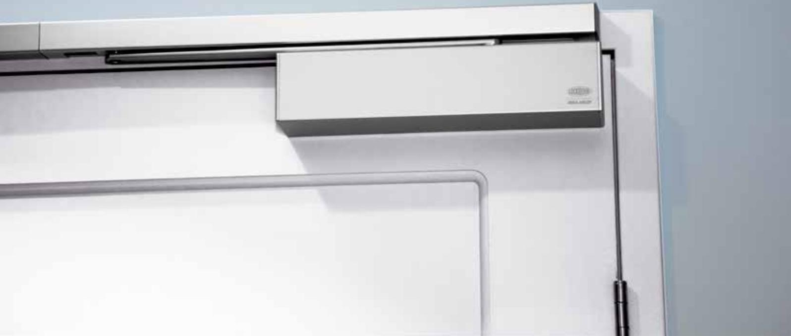
The Lockwood 2616EMC is a small single door electromechanical hold open device system with a sliding arm. It is applicable for places, where fire doors are constantly kept open. The door is kept open at a selected angle. If fire breaks out, the door is closed, preventing smoke and flames from spreading. Applications for 2616EMC include hotels, office buildings and other fire doors where hold open function is needed.
